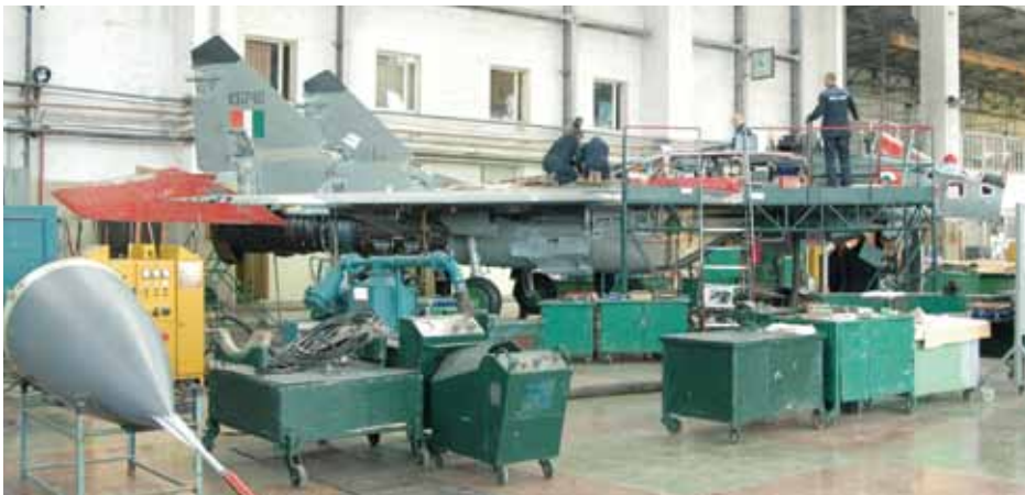
Indian AF MiG-29s under overhaul and modernization at MAPO plant
