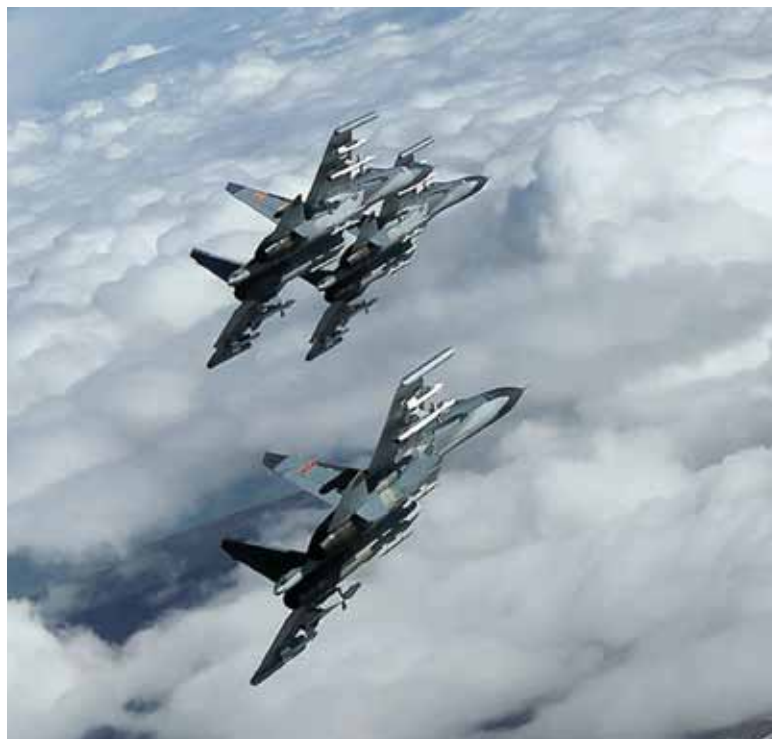
Example of "licensed copying" is the Chinese J-11 fighter jet, based on Russia's Su-27
